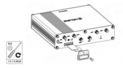
2. Antenna Installation. Rotate the antenna into the antenna connector accordingly.
