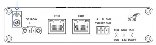
**6. Connect the router to the computer.** Connect the Ethernet cable to any port labeled ETH0 or ETH1 of the router, and connect the other end of the cable to your computer.
