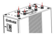
**3. Terminal Block Installation.** Insert the 3-PIN or 4-PIN terminal blocks into the interfaces connector, then can connect the devices or sensors to the router via corresponding interfaces.
