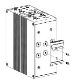
**6. Wall Mounting.** Use 4 M3 screws to fix the Wall Mounting kit to the device.
