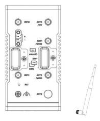
**3. Terminal Block Installation.** Insert the 4 PIN,5PIN and 6PIN terminal blocks into the interfaces connector, then can connect the devices or sensors to the gateway with wires via corresponding interfaces.
