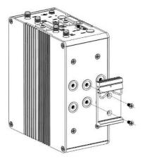
**6. Wall Mounting.** Use 4 M3 screws to fix the Wall Mounting kit to the device.
