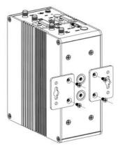
**7. Grounding the Device.** Grounding will help to prevent the noise effect due to electromagnetic interference (EMI). Connect the device to the site ground wire by the grounding screw before powering on.
