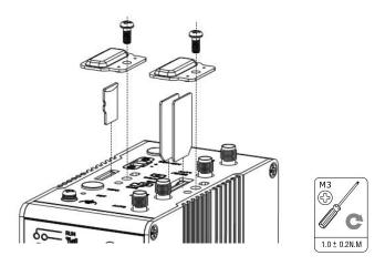
2. Antenna Installation. Rotate the antenna into the antenna connector accordingly.
